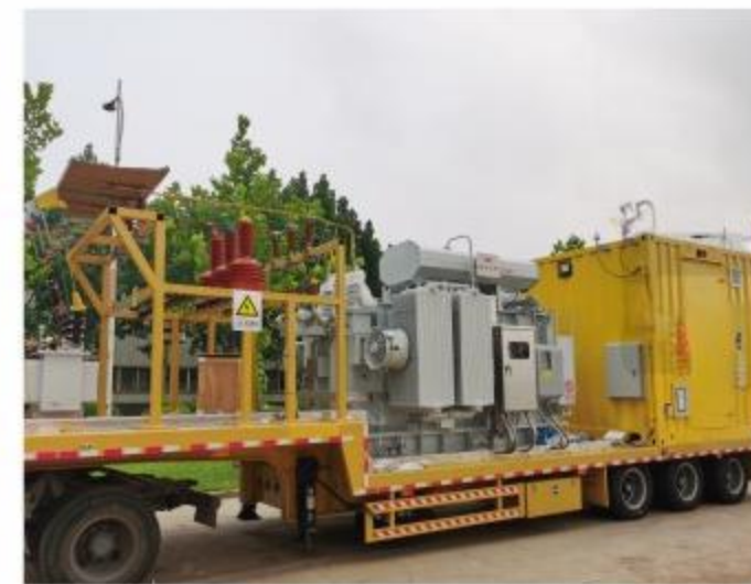
国网青海海东供电公司车载变 Vehicle-mounted Mobile Transformers of State Grid Qinghai Haidong Power Supply Company
